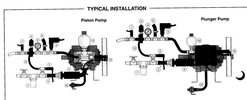
It is recommended that a secondary protective device such as the *CAT PUMP Pop-Off Valve* be installed to assure pump protection should the regulator malfunction. Refer to Troubleshooting for more information on malfunction of regulator.
